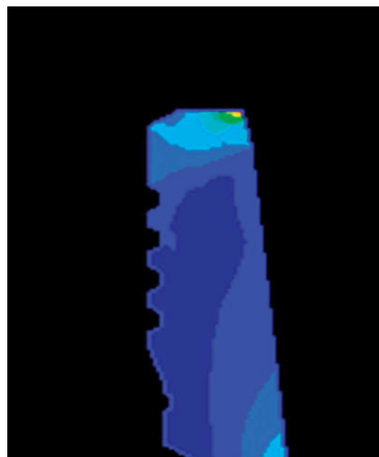
Figure 7 - Morse taper implant cervical region under axial load of 100 N.
