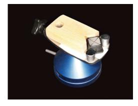
Figure 1. Articulator table with white adhesive, wooden device and tip with acrylic resin and mark.
