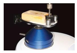
Figure 5. Implant being placed into the resin.
