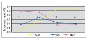
GRAPH 1 - Graph showing the initial movement of the first molar (anteroposterior direction) at points in the palatal (1) and mesiobuccal (2) roots, and at mesial (3) and distal (4) points of the tube bonded to the crown, as observed in all three computer simulation models (ACR, CR and BCR).
