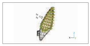
FIGURE 13 - Boundary conditions resulting from the application of force to the center of resistance (CRes).
