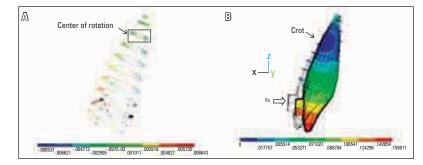
FIGURE 8 - Axial stress (N/mm<sup>2</sup>) resulting from a 0.70 N load.
