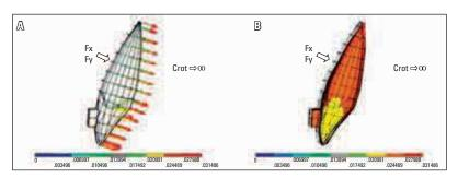
FIGURE 15 - Translatory movement resulting from the application of force to the center of resistance (CRes): A) resulting vectors, B) resulting displacement.
