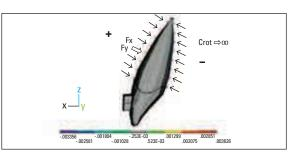
FIGURE 14 - Axial tensions (N/mm<sup>2</sup>) resulting from force applied to the center of resistance (CRes).
