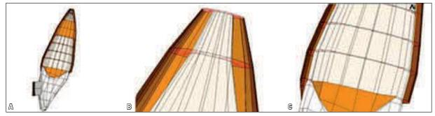
FIGURE 2 - Finite element model with the periodontal fibers connecting the tooth and alveolus.
