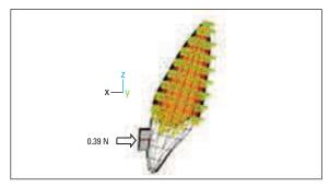
FIGURE 4 - Boundary conditions applied to the model: force of 0.39 N in the bracket and restrictions to alveolar movements.
