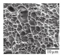
FIGURE 2 - Fractograph of Ø 0.9 mm wire that underwent tensile testing in different magnifications: A) surface of wire fracture; B, C) enlargement of region shown in (A).
