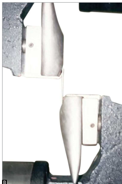
Figure 1 - A) Machine used on the performance of traction resistance tests, B) Detail of the wire tied by its ends to the machine's nails, C) Device used on the performance of tests at oral temperature ( 37^\circ\text{C} ).
