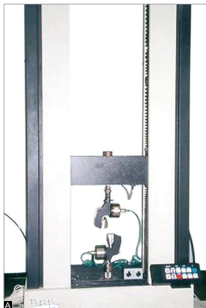
Figure 1 - A) Machine used on the performance of traction resistance tests, B) Detail of the wire tied by its ends to the machine's nails, C) Device used on the performance of tests at oral temperature ( 37^\circ\text{C} ).
