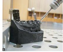
Figure 2 - Coordinate measuring machine (CMM). A) Device setting general view. B) Dental casts are placed to have CBPs digitized by the touch probe of the CMM.
