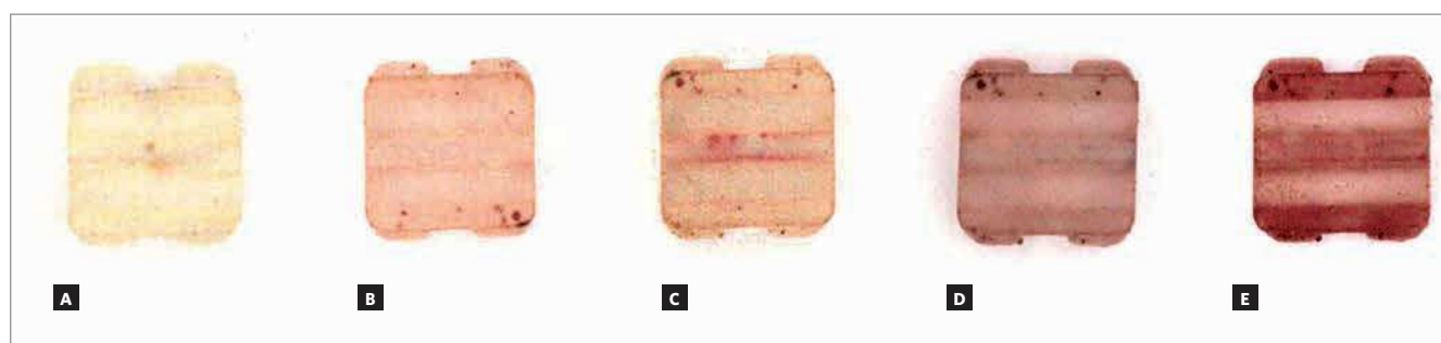
Figure 1 - Brackets after immersion in red wine: A) baseline, B) after 24 hours, C) after 72 hours, D) after 7 days, and E) after 14 days of immersion.
