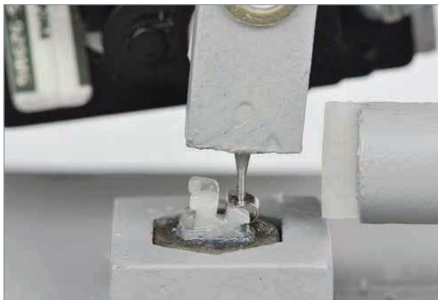
Figure 3 - Adapted devices recommended by the manufactures for clip opening and closure.
