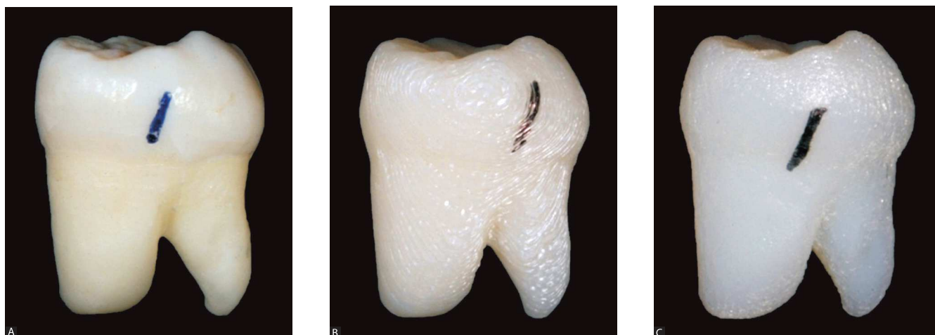
Figure 2 - A) Original tooth. Replicas: B) tooth printed by the fused deposition modeling method (FDM) and C) tooth printed by the PolyJet method. (Source: Lee et al, 2 2015).
