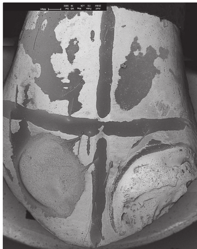
Figure 3 - Control sample: In upper left quadrant, etching; in upper right quadrant, etching + bonding agent; in lower left quadrant, etching + bonding agent + conventional resin; in lower right quadrant, etching + bonding agent + pigment resin.
