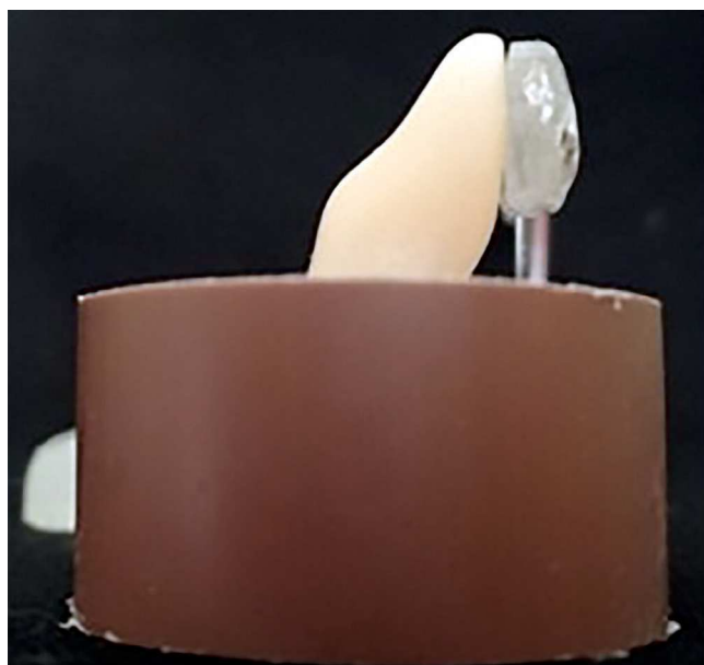
Figure 1 - Image of the positioner used to guide the tooth position.
