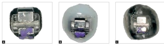
Figure 1 - Original bracket (A), bracket with resin pad (B), bracket with a metal pad (C).
