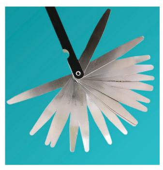
Figure 7 - Feeler gauge to measure the amount of separation at teeth contact point.
