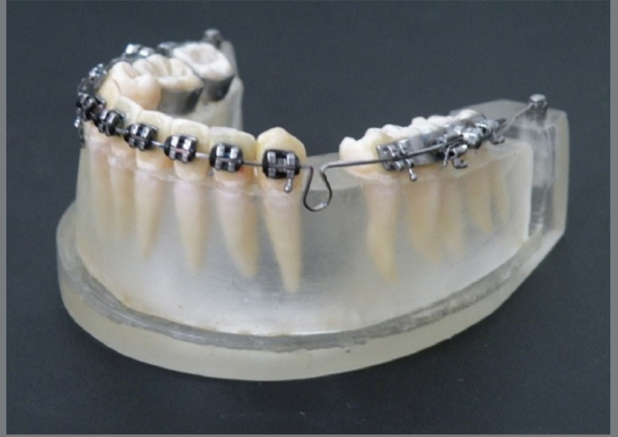
Figure 2: Teardrop loop spring test specimen.
