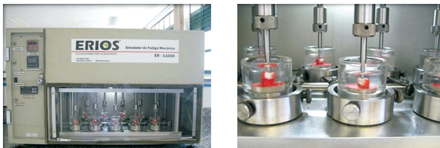
Figure 3. Samples in Mechanical Fatigue Machine (ERIOS) submitted to action of vertical forces.
