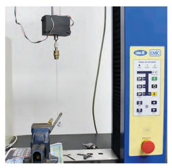
Figure 2. Cantilever bending test using a universal testing machine.
