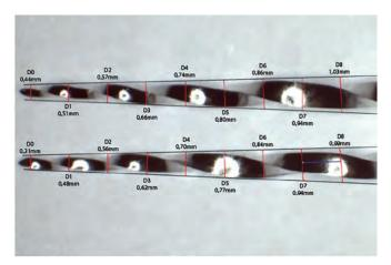
Figure 1. Taper measurement at D0, D3, and D6 using the TSView software.
