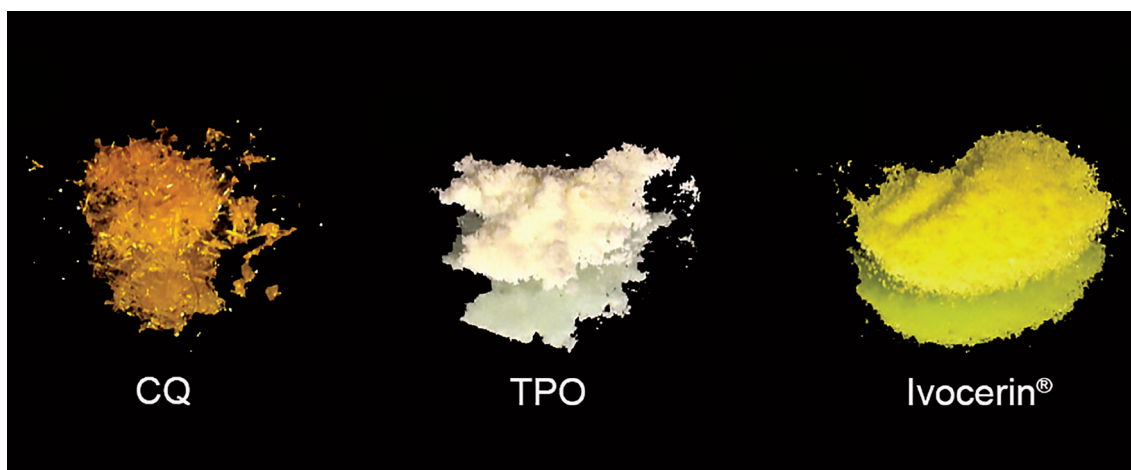
Figure 1: Photoinitiators used in dental materials: camphorquinone (CQ), trimethylphosphinic oxide (TPO) and benzoyl germanium (Ivocerin®).
