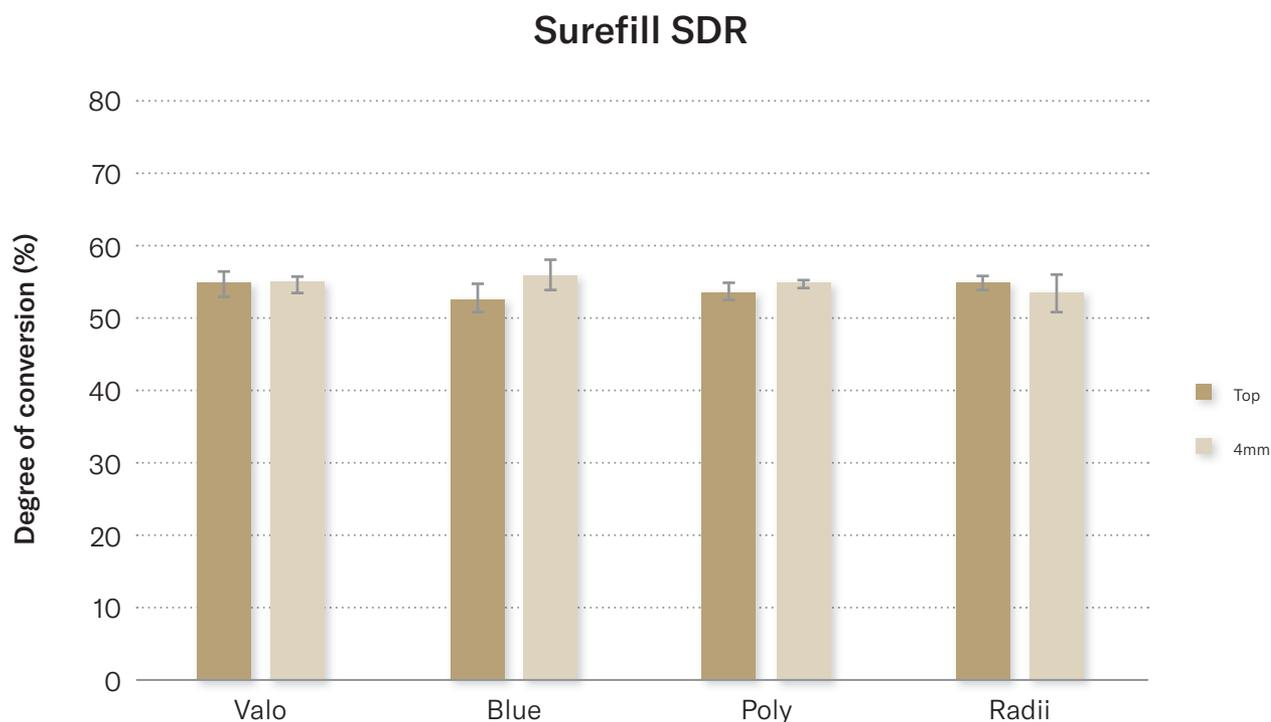
**Figure 3:** DC to 0.1 mm (representing top) and 4 mm thickness samples of Surefill SDR resin when photoactivated by four LCU.
