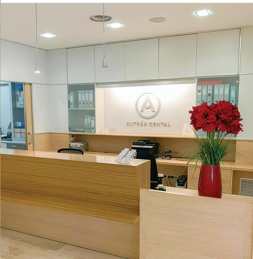
The central element is the reception desk, giving private access to the service areas and the administration office. The counter consists of a vertical inclined plane and a horizontal work plane. The inclined vertical plane allows greater physical proximity between the patient and the reception staff.
