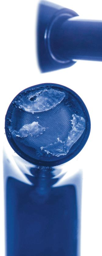
→ Figure 1: Dirtiness and resin-based material residues adhered to the light curing units' tip must be removed. A gauze dipped in isopropyl alcohol can be used for that.
